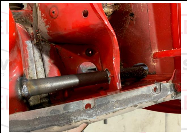
PHOTO 9 ATTACHMENT TO FRONT SUSPENSION
