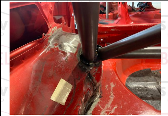
PHOTO 5 REAR BACKSTAY TO BODYSHELL ATTACHMENT
