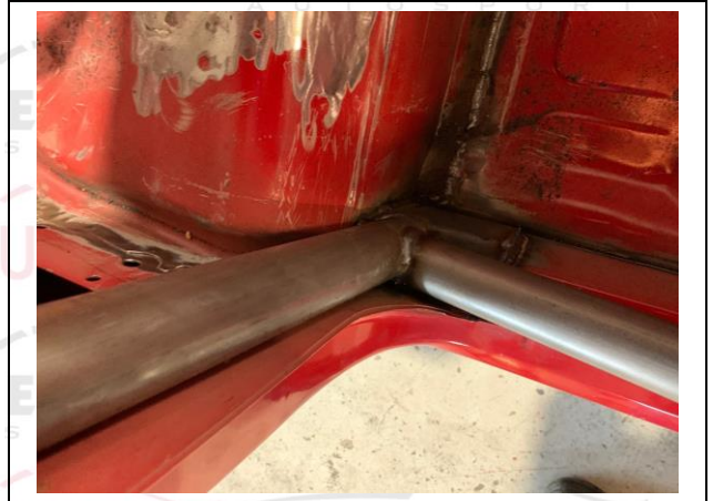
PHOTO 6 FRONT ROLLBAR TO FLOOR ATTACHMENT
