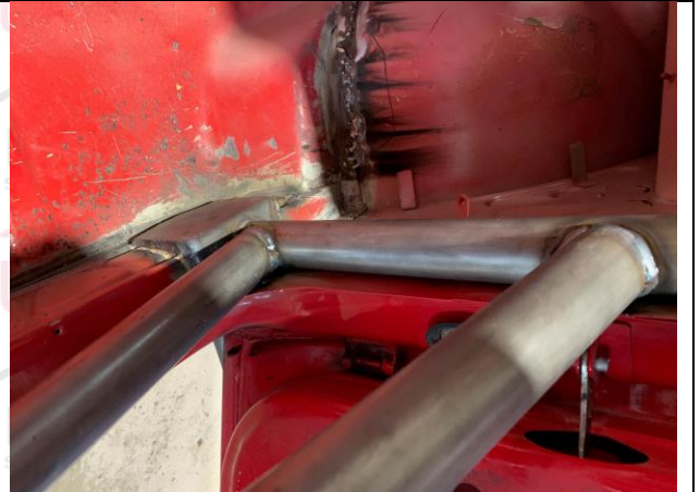
PHOTO 4 MAIN ROLLBAR TO FLOOR ATTACHMENT
