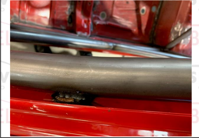
PHOTO 7 FRONT ROLLBAR TO "A" PILLAR ATTACHMENT
